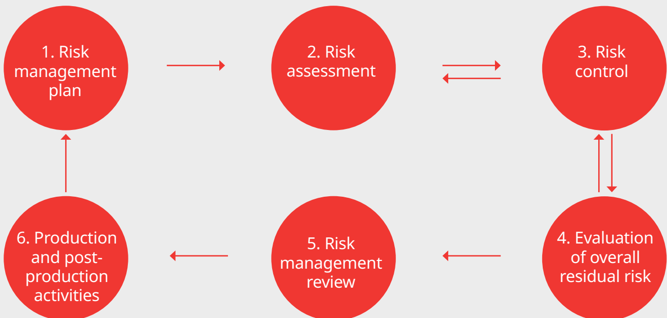
Figure 1 – The six process steps in the risk management process of BS EN ISO 14971 [1].
