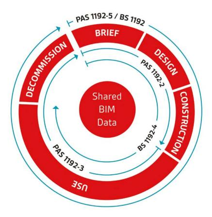
The diagram shows how PAS 1192-2 outlines the requirements for BIM Level 2 for the design and construction phase of a project, while PAS 1192-3 outlines the requirements for the specification, production and management of information during the 'in use' phase of the asset. It will typically be in this phase that the vast majority of savings from a BIM-led project will be made, because of its potentially lengthy duration (often 20 years or more).
