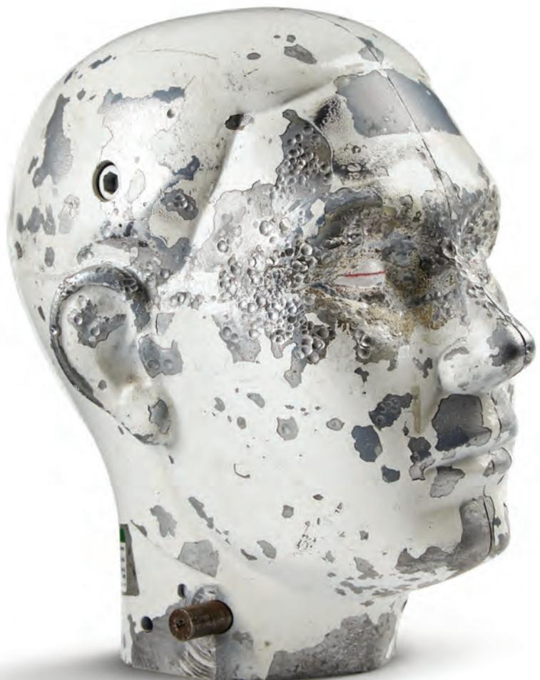
To test protective eyewear we fire a 6mm ball bearing at up to 190 metres per second (425mph) at a head form like this. This helps a wearer's eyes remain protected in the most dangerous environments.
