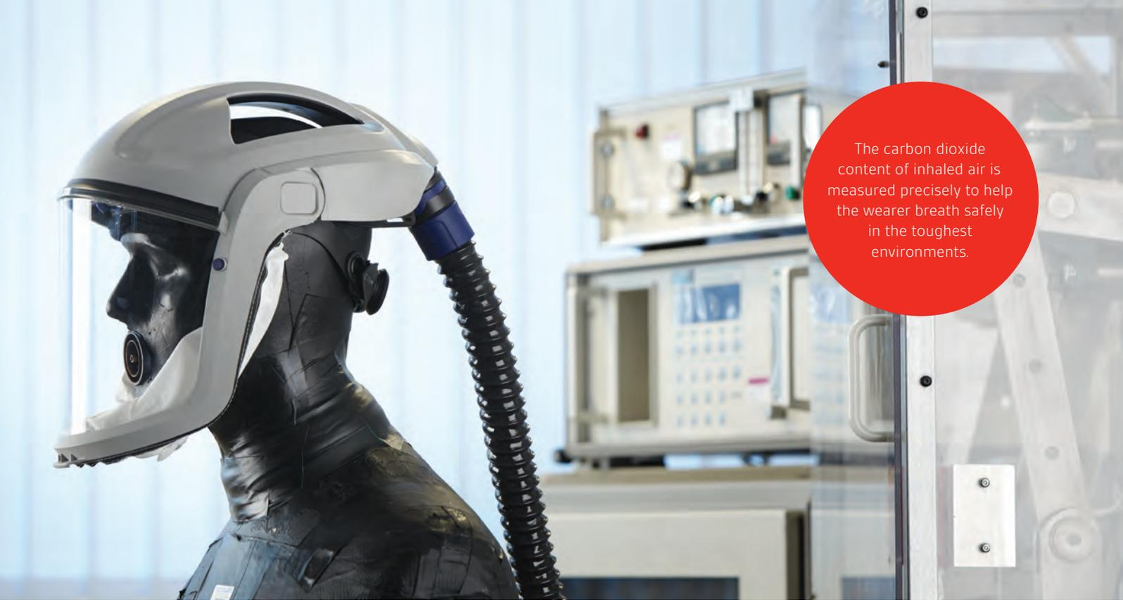
The carbon dioxide content of inhaled air is measured precisely to help the wearer breath safely in the toughest environments.
