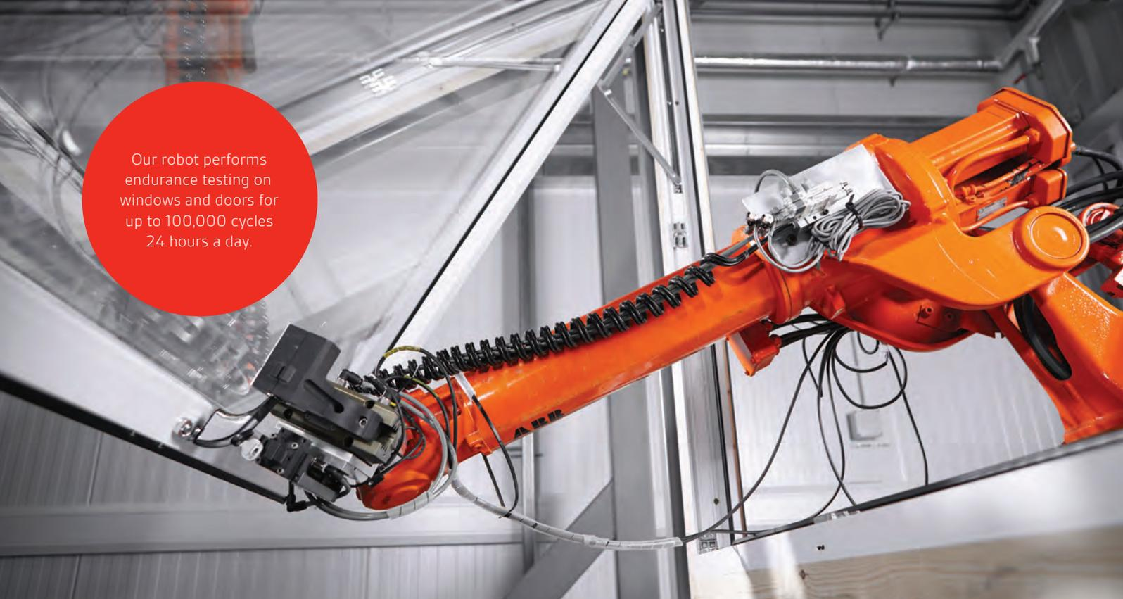
Our robot performs endurance testing on windows and doors for up to 100,000 cycles 24 hours a day.
