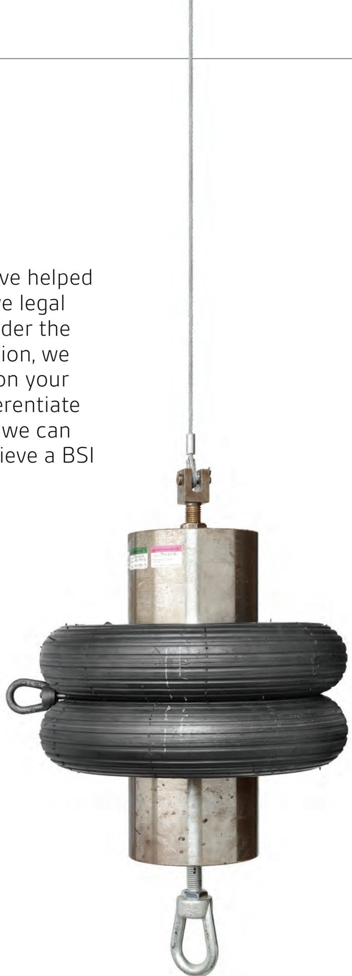
The pendulum impact test makes sure toughened and laminated glass breaks safely, preventing serious injuries such as lacerations and piercing.
