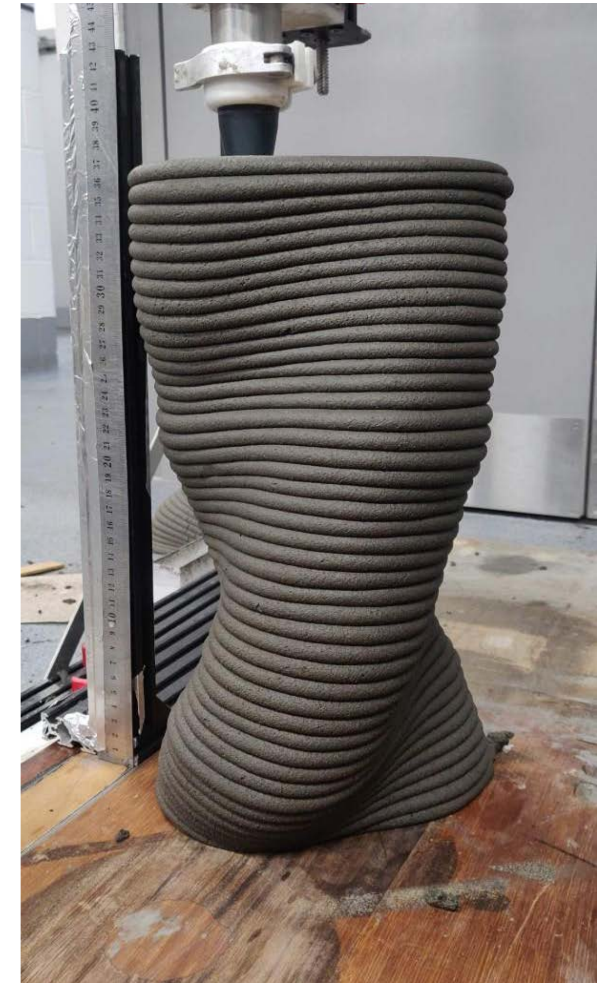
Figure 2 – an example of 3D printed building block using low-carbon concrete by AMTC research group
