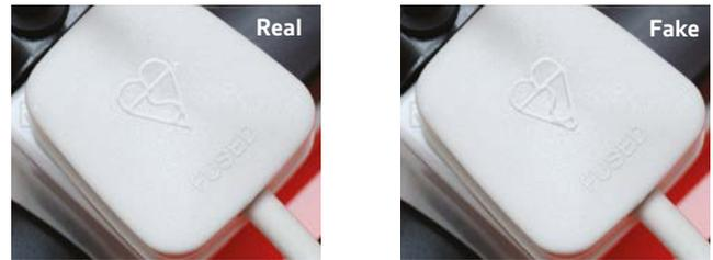
In addition, the licence number on the 'Approved by' stamp should start with the letters KM and consist of five or six numbers, usually between 1 and 9. A series of zeroes means zero — no licence, no certificate, no BSI approval. If you're an appliance manufacturer and distributing small electrical accessories that way, you should also check that
