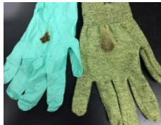
Picture of 25-101 underglove & 80-813 overglove after folded glove flame test – visual marks only, no burn holes
