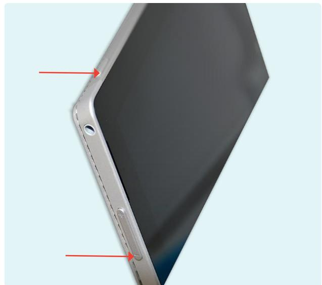
**Note:** The power and volume locations vary between Surface tablet models. The above is a Surface Pro 3.
