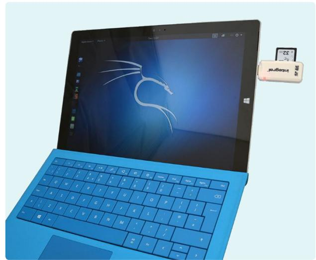
Boot the Surface tablet with the USB stick inserted and it should boot straight into Kali2 Linux.
