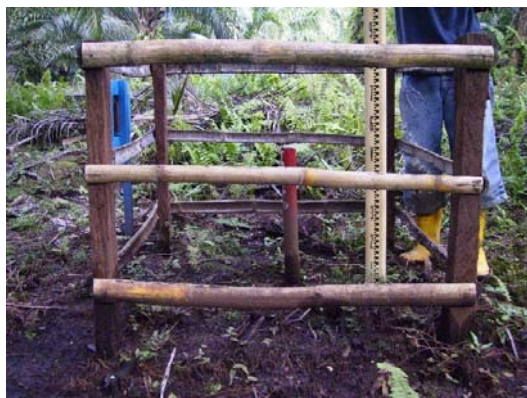
Plate 3: Survey Point for Monitoring Peat Subsidence
